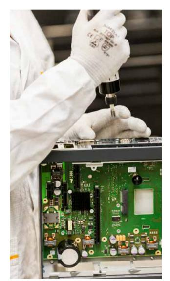
The fastening torque of screws is defined and monitored.
