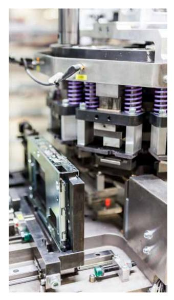
During production, the housing of the Panel PC 2200 is customized to match the configuration.
