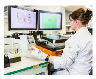
100% of circuit boards are subjected to in-circuit testing, where each electrical circuit is contacted and measured.
